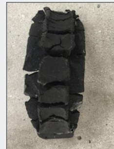
Bentonite waterstops can disintegrate over time while Krytonite will continue to stop water.
